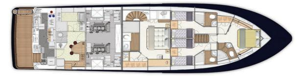
THE ELD FULL (EXTENDED LOWER DECK FULL) LAYOUT HAS ALSO TWO ACCESSES TO THE LOWER DECK — ONE TO THE GUESTS AND ONE TO THE MAIN SUITE. WITHOUT THE CENTRAL CORRIDOR IN THE LOWER DECK BOTH THE MIDSHIP STATEROOMS ARE WIDER. THERE IS NO FISHING DECK PROVIDING MORE SPACE IN THE LOWER DECK STATEROOMS.
